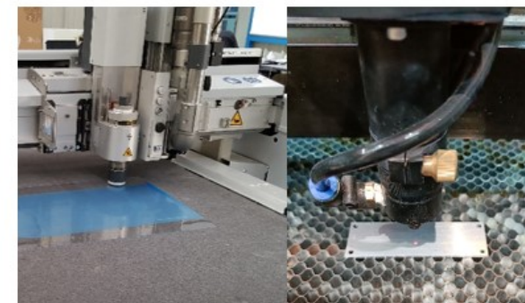
Cutting (mechanical & laser)
